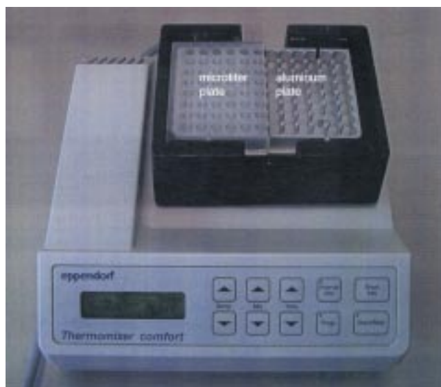
Figure 5. Commercially available Eppendorf shaker with a modified aluminum plate on which the microtiter plate is placed (for better visualization half of the Al plate is uncovered). [61,63]
