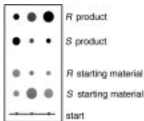
Figure 11. Schematic representation of a TLC plate showing the result of kinetic resolution of a rac -starting material. [72]
